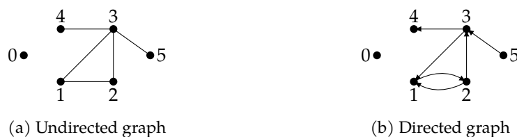
Figure 8.1: An undirected graph and a directed graph on the vertex set V = \{0, 1, 2, 3, 4, 5\} .
