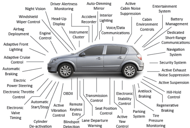
Figure: Features requiring MCUs in a car. Source: https://www.popsautoelectric.com/tag/automotive-trouble-lights/
